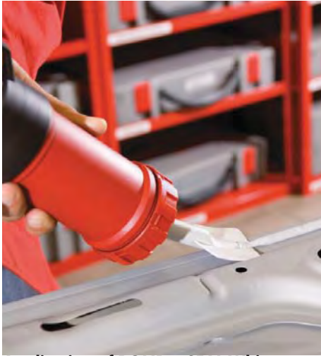
Application of BOND + SEAL White on new panel, with Flanged Seam Nozzle.
